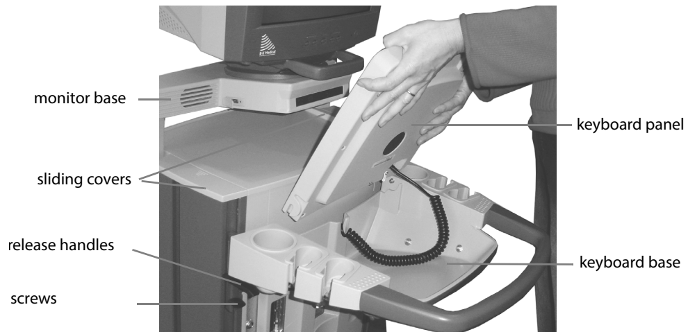
Figure 4-5. Removing the keyboard base.
