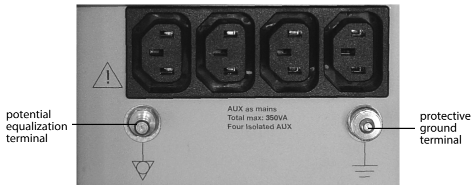
Figure 4-4. Auxiliary power outlets.
